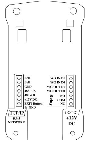
the base case is made by ZINC or plastic ( By selection) And RJ45 Port is disable for the BF5
